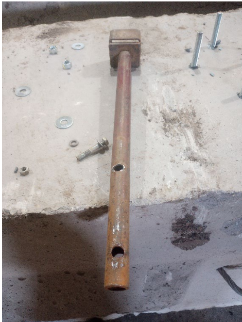
Water Main Line Key Fabrication
