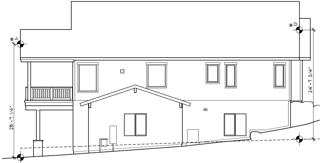
Figure 3: Original Building Heights on Right Elevation
